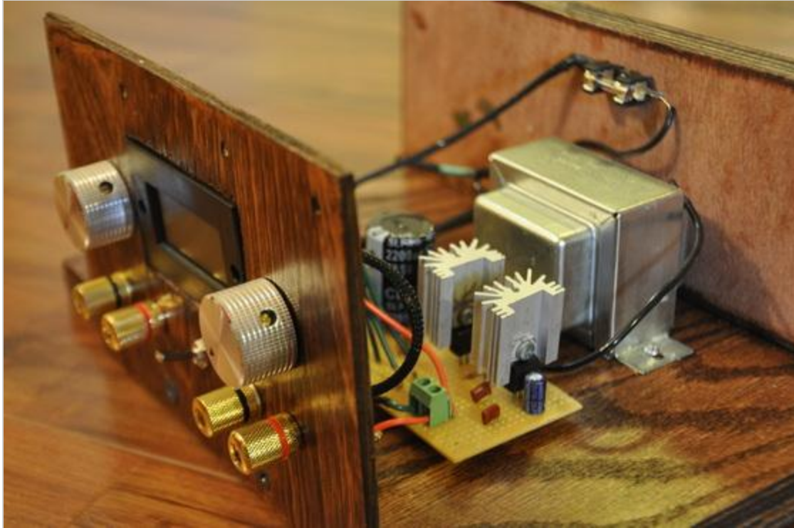
Power supply during chassis construction
